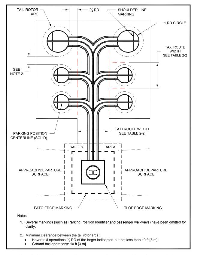
Figure 2-18. Parking Area Design - "Back-out" Parking Positions: General Aviation
