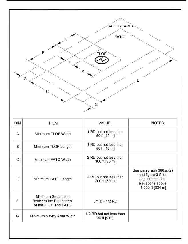
Figure 3–2. TLOF/FATO Safety Area Relationships and Minimum Dimensions: Transport
