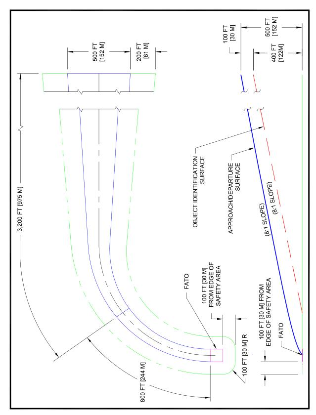
Figure 4–33. Airspace Where Marking and Lighting are Recommended: Curved Approach: Hospital
