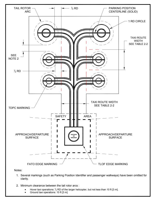
Figure 2-17. Parking Area Design - "Turn-around" Parking Positions: General Aviation
