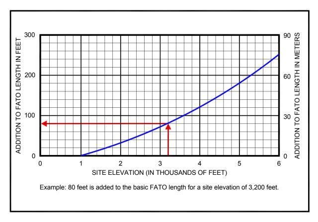
Figure 4-4. Additional FATO Length for Heliports at Higher Elevation: Hospital
