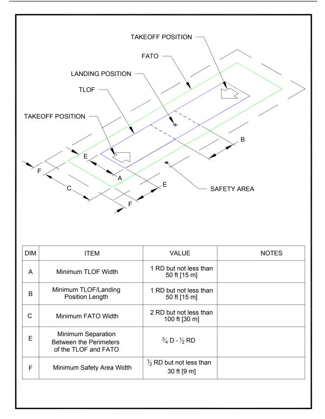
Figure 3-3. Elongated FATO with Two Takeoff Positions: Transport
