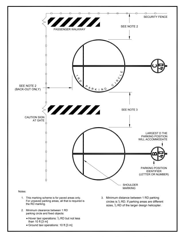
Figure 2-20. "Taxi-through" and "Back-out" Parking Position Marking: General Aviation
