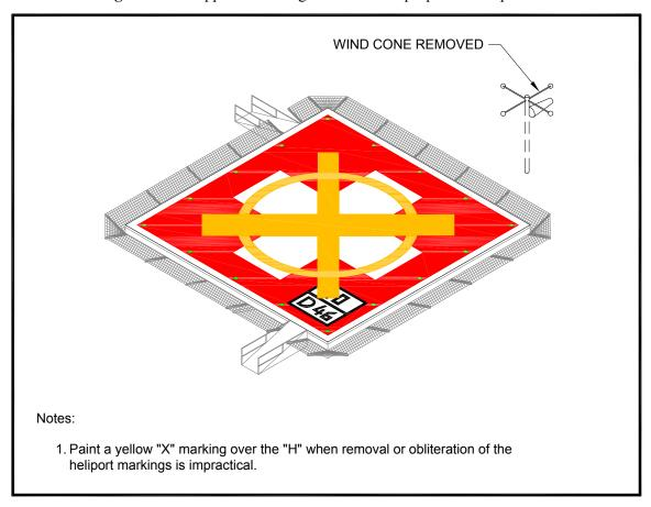
Figure 4–27. Marking a Closed Heliport: Hospital
