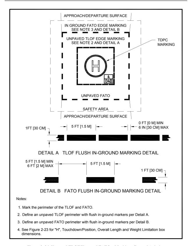
Figure 2-26. Unpaved TLOF/Unpaved FATO - Marking: General Aviation
