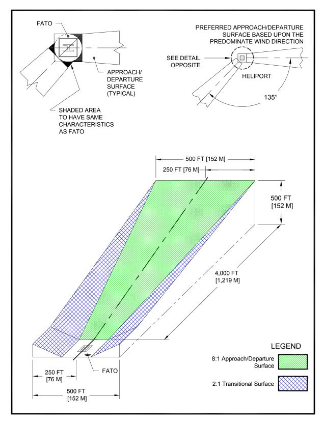
Figure 3–7. VFR Heliport Approach/Departure and Transitional Surfaces: Transport
