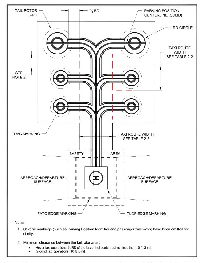
Figure 4-16. Parking Area Design - "Turn-around" Parking Positions: Hospital
