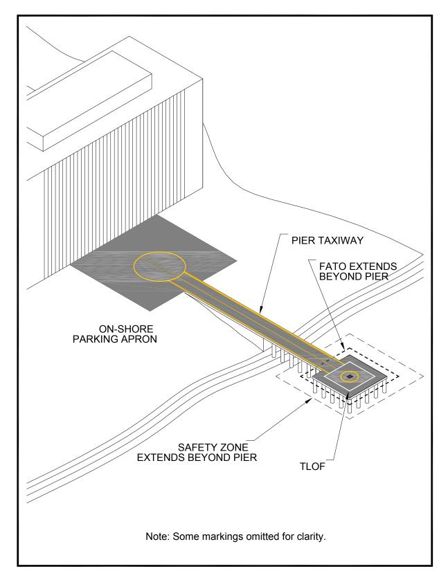
Figure 2-6. Non-load-bearing FATO and Safety Area: General Aviation
