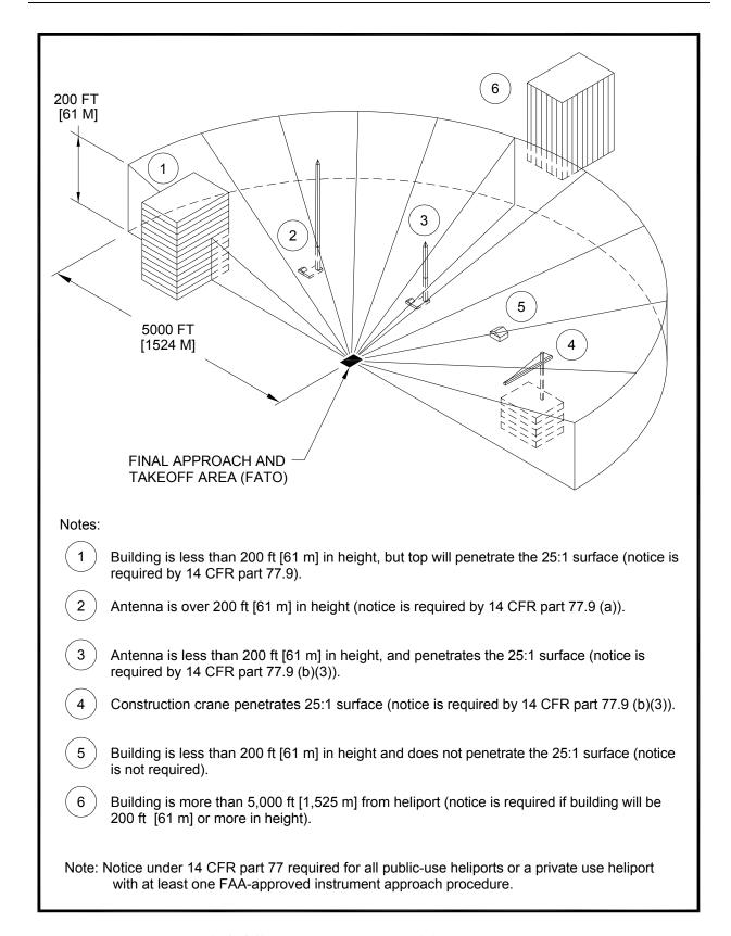
Figure 1-4. Offsite Development Requiring Notice to the FAA
