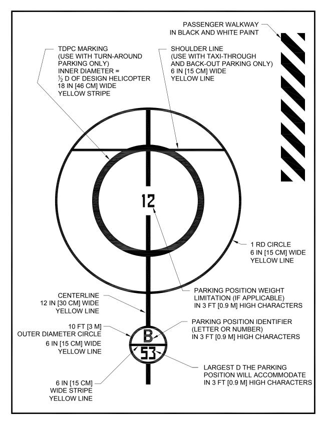
Figure 4-20. Parking Position Identification, Size, and Weight Limitations: General Aviation
