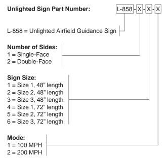
Note: To order a sign that will be stake-mounted, add "-S" to the end of the part number (e.g., L-858-1-1-2-S). (A stake-mounted sign is not ETL certifiable.)
